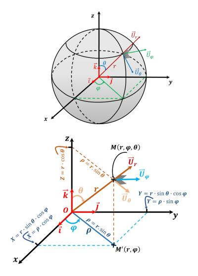
The conversion between Cartesian coordinates (x, y, z) and spherical coordinates  $(r, \theta, \varphi)$  is given by the following equations:
